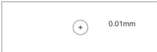
2) Firstly, Put the scale under the lens. Adjust the lens to max magnification 5X (Adjust the **zoom body hand wheel 1**). Then adjust **focus holder hand wheel 2** to suitable working distance(Standard working distance is about 86mm).Let the image become clearest.
